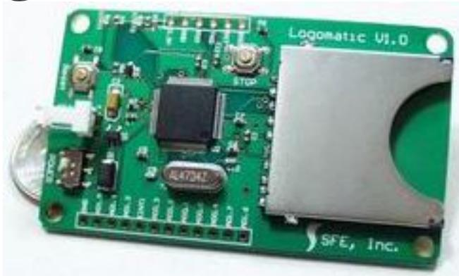
This wind logger project was designed to help a friend who wants to log wind speed for one year. It uses an inexpensive cup anemometer from Biral (see photo, left) available here in the UK. The anemometer contains a reed switch with rotating magnets which produce two switch closures per revolution of the cup assembly. It can be connected to produce a varying frequency output, whose frequency 0 - 100Hz corresponds to windspeeds of 0 - 40m/s.
